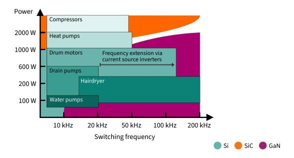
It is possible to reduce the size of passive components, including the heatsink, in many cases. These improvements allow the inverter to simultaneously increase efficiency, reduce its overall dimensions, and maintain cost competitiveness with traditional designs.
